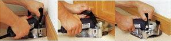
UNDERCUTS INSIDE CORNERS, TOE SPACES AND ALONG WALLS.
