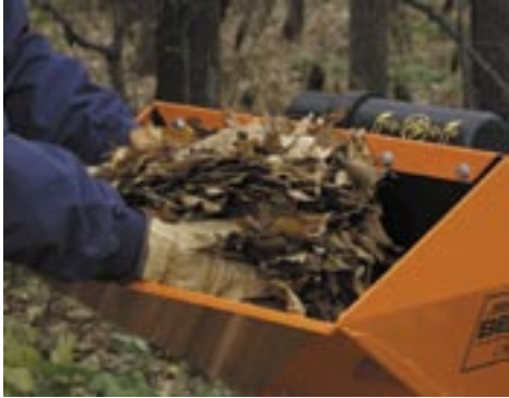
Leaves can be quickly disposed of with the large shredder hopper.
