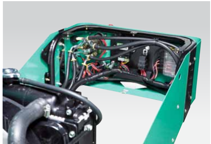
Swing-away upper frame design makes service and maintenance easy.
