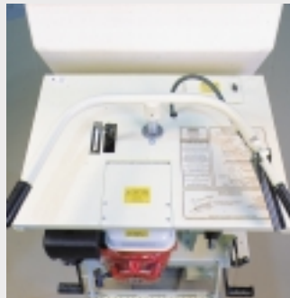
Control panel has smoother, cleaner surface due to fewer controls. Redesigned handlebar is more rigid and incorporates a heavy-duty cast aluminum "dead-man" brake.
