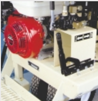
Operating and parking brake assembly is foot-actuated.
